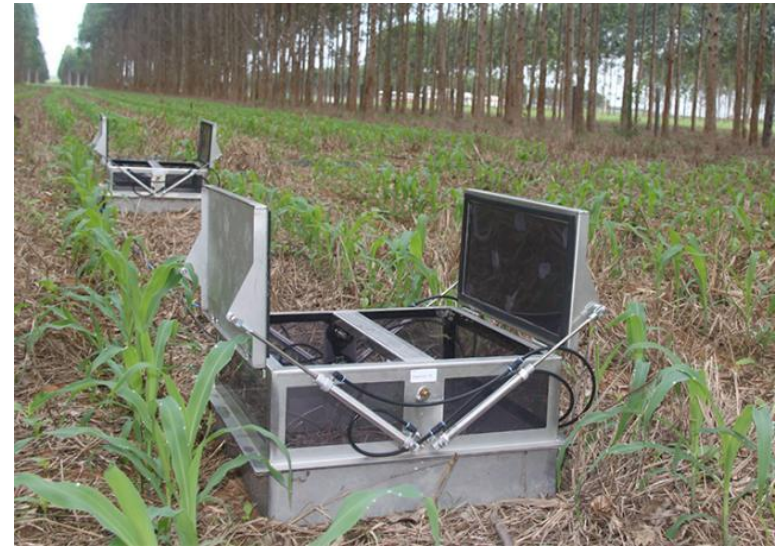
Automatic GHG collection and analysis system, installed in the ILPF experiment at Embrapa Agrossilvipastoril, Sinop-MT
