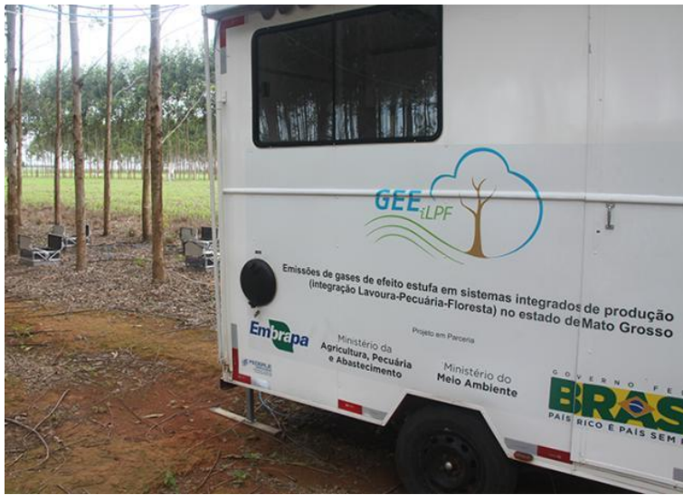
Automatic GHG collection and analysis system, installed in the ILPF experiment at Embrapa Agrossilvipastoril, Sinop-MT
