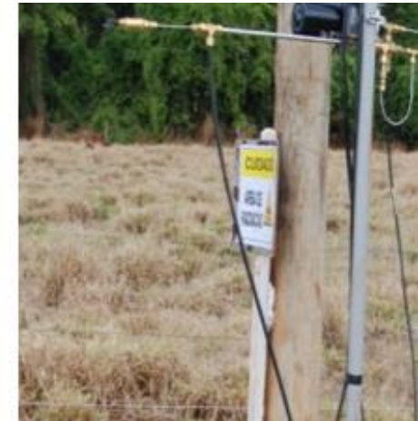
Micrometeorological system for monitoring the emission of N 2 O e CO 2
