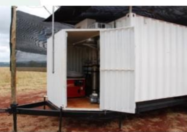
Micrometeorological system for monitoring the emission of N 2 O e CO 2
